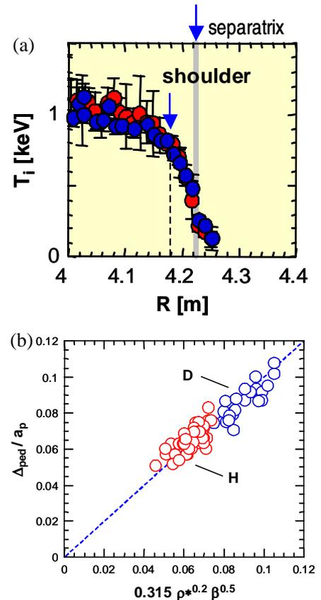
**Figure 4.** (a) Pedestal  $T_i$  profiles for deuterium and hydrogen plasmas at the same  $\beta$  and  $v^*$ . (b) Scaling of H-mode pedestal width obtained by dimensionless transport experiment.
