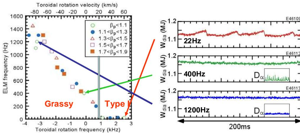
**Figure 2.** Relation between ELM frequency and toroidal rotation in type-I and grassy ELMs. Time evolutions of plasma stored energy for the cases of toroidal rotation in co, balanced and counter.
