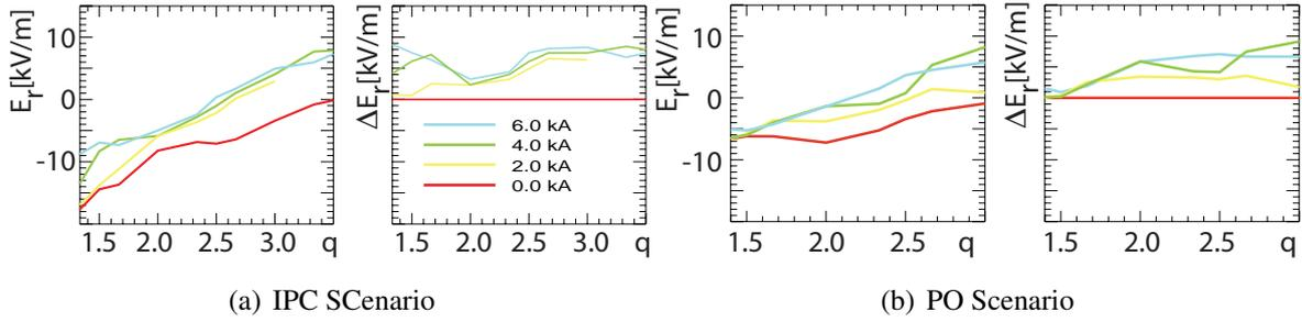
**Figure 3:** Radial profiles of the radial electric field and its changes due to the RMP .
