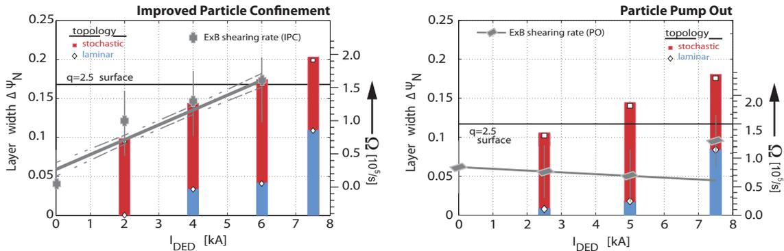
**Figure 4:** Comparison of  $\Omega$  with the evolution of the magnetic topology (during IPC & PO).
