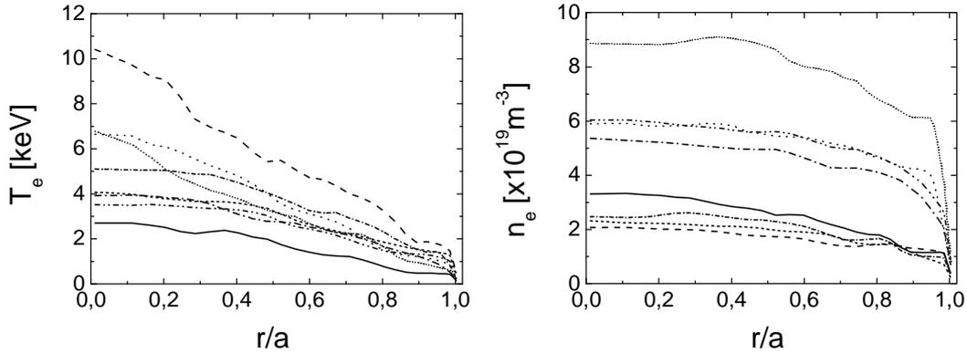
**Figure 1.** Electron density and temperature profiles obtained from the LIDAR Thomson scattering and electron cyclotron emission diagnostics used in the UTC simulations to test different JET discharges. One  $T_e$  and one  $n_e$  profile has been used for each point in Figure 4.
