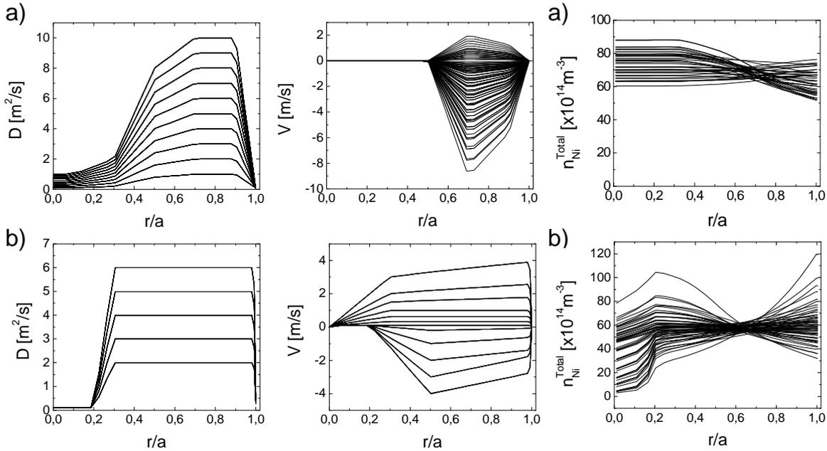
**Figure 2a), b)** Sets of the diffusion  $D(r)$  and convection  $v(r)$  transport coefficients used in simulations as an unknown discharge parameter in the region where the Li-like emissions is coming from.
