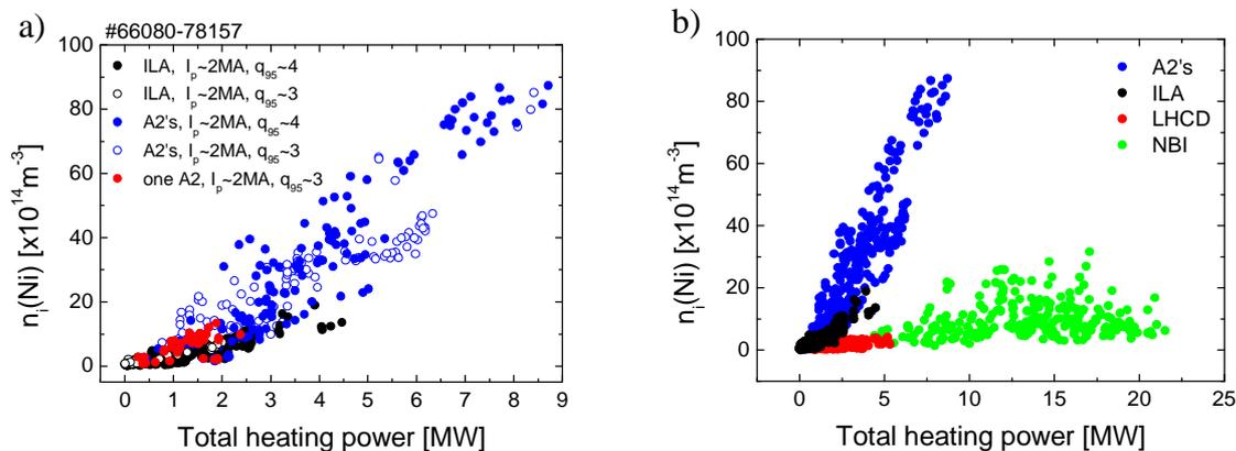
**Figure 5.** Correlation between the derived Ni densities ( $r \sim 0.5-0.6$ ) and applied heating power for a) the RF heating systems. b) the different JET heating systems.
