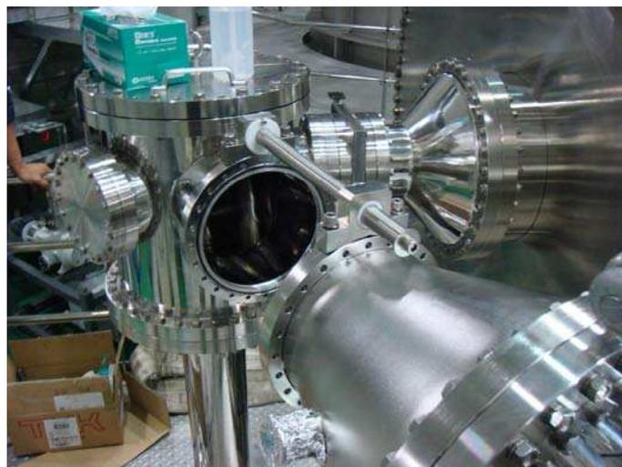
*Fig. 4. A detail view of the XICS on the KSTAR pump duct.*
