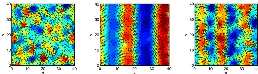
Figure 1: Snapshot of potential  $\phi$  in the saturated quasi-stationary turbulent state for three related models: (left) HW defined by equations 1 where zonal flows are damped; (centre) MHW defined by equations 2 allowing the self-generation of zonal flows; (right) intermediate state of MHW where total kinetic energy of zonal flows is set equal to that of non-zonal drift wave turbulence at each time step.
