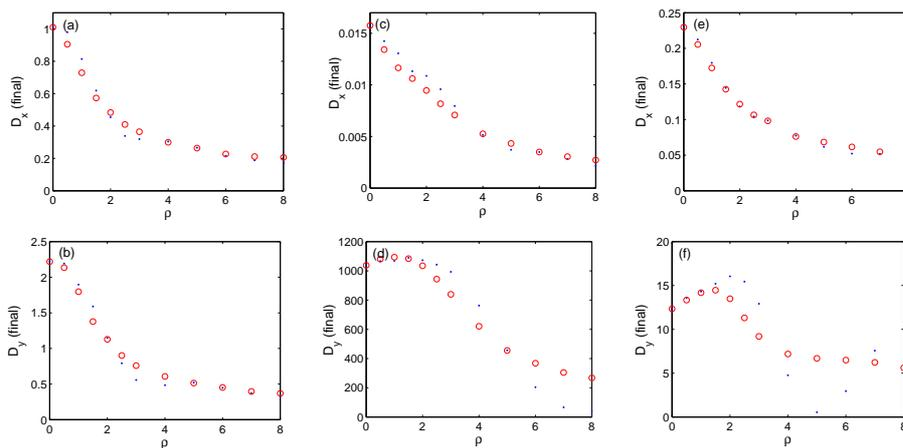
Figure 3: Value of diffusion coefficients  $D_x$  and  $D_y$  at the end of the simulation ( $t = 2500$ ) as a function of  $\rho$ : (a) and (b) HW case; (c) and (d) MHW case; (e) and (f) intermediate turbulence case. Blue dots indicate results when all the test particle share the same Larmor radius  $\rho$ ; red circles indicate results when the Larmor radii are distributed around a most probable value  $\rho$ .
