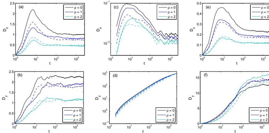
Figure 2: Running diffusion coefficients  $D_x$  and  $D_y$  versus time: (a) and (b) HW case on a log-linear scale; (c) and (d) MHW case on a log-log scale; (e) and (f) intermediate turbulence case on a log-linear scale. The value of  $\rho$  is indicated by the colour of the plotted lines. Full lines indicate results when all the test particle share the same Larmor radius  $\rho$ ; dashed lines indicate results when the Larmor radii are distributed around a most probable value  $\rho$ .
