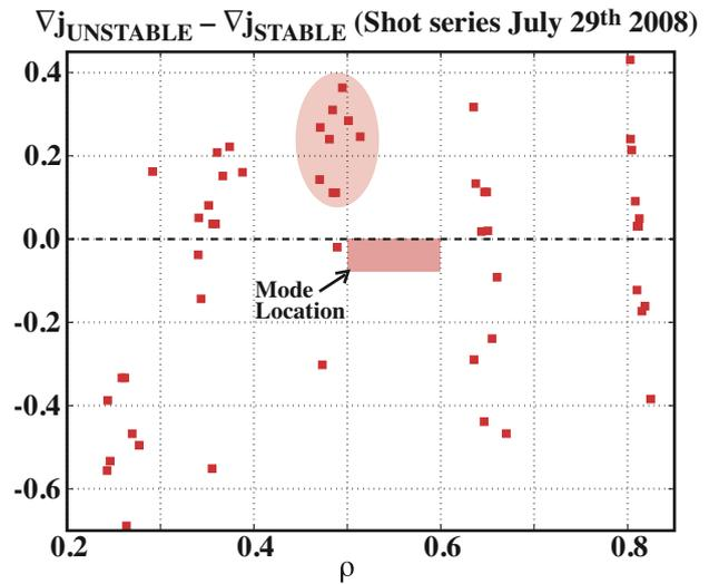
Fig. 3. Differences between local current gradients of unstable discharges at the time of the mode onset, and of stable discharges at the same time slice. The shaded area highlights the series of  $\nabla j_{unstable} > \nabla j_{stable}$ .
