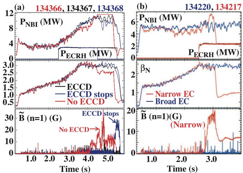
Fig. 1. Evolution of NBI and EC power (first row),  $\beta_N$  (second row),  $n=1$  MHD activity by Mirnov coils signals (third row) for cases with different ECCD (a) timing (b) deposition width.
