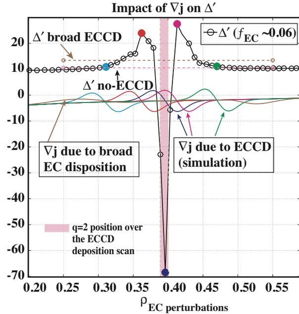
FIG. 4.  $\Delta'$  values for all simulated ECCD depositions (black  $f_{EC} \sim 0.06$ , brown broad  $f_{EC}$ , pink no ECCD) and  $\nabla j$  for ECCD depositions around the  $q=2$  rational surface. The coloured circles correspond to the matching colour for the  $\nabla j$  trace.
