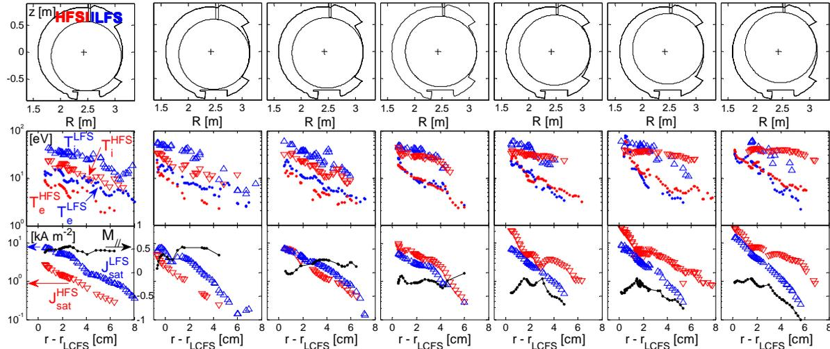
Fig. 6. Radial profiles of  $T_i$ ,  $T_e$ ,  $j_{sat}$  and  $M_{||}$  measured in seven RFA reciprocations in the discharge with steadily displaced outboard contact point. HFS / LFS indicate the side of the RFA. For  $M_{||} > 0$  the flow is directed towards the LFS analyzer.
