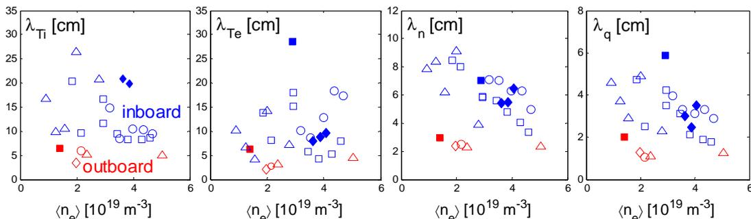
Fig. 3. The e-folding lengths of  $T_i$ ,  $T_e$ ,  $n_e$  and  $q_{||}$  plotted against the volume-averaged plasma density. Inboard / outboard indicate the contact point. Symbols correspond to poloidal cross sections from Fig. 1. Full symbols: detached discharges.  $\lambda_{T_i}$  for two detached discharges is almost infinite and does not appear on graph.
