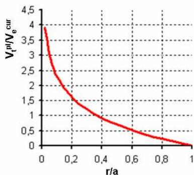
Fig.1 The ratio of plasma toroidal rotation velocity (eq. (5)) to the current electron velocity versus of effective minor radius.
