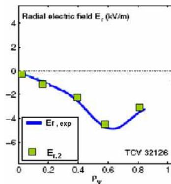
Fig.2 An estimation of radial electric field profile  $E_r(r)$  in a typical ohmic discharge in the TCV plasma [3]: the  $E_{r,exp}$  is experimental profile in the discharge, the  $E_{r,2}$  is calculated by eq. (7).
