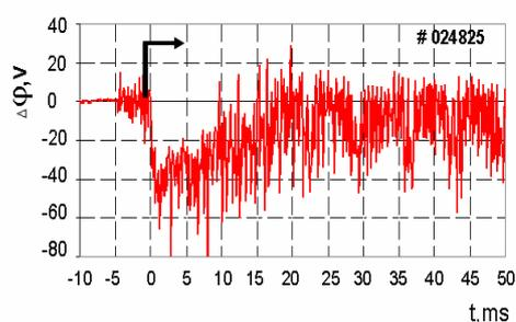
Fig.3 Time dependence of the T-11M tokamak chamber electric potential during the discharge.
