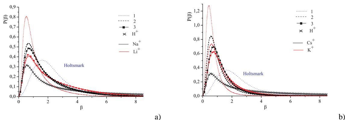
**Figure 3:** Comparison of EMD calculations in a frame of the Hellmann-Gurskii-Krasko pseudopotential model for  $H^+$ , (a)  $Li^+$ ,  $Na^+$  and (b)  $K^+$ ,  $Cs^+$  plasmas at  $T = 30000K$  and  $\Gamma = 2$ . 1: EMD with RDF (13) obtained from the screened HGK in Debye approximation (20) in [1]; 2: EMD with RDF obtained from the screened HGK in the moderately coupled approximation (11-14) in [1]; 3: Monte Carlo simulations (MC).
