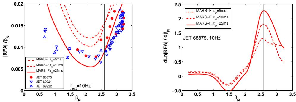
Figure 2: (a) Comparison of the modelled RFA amplitude (curves) with the experimental data (dots) from three similar pulses. Various values of the wall penetration time are assumed in the modelling. The solid vertical line indicates the computed no-wall beta limit. (b) Agreement between the logarithmic RFA threshold and the no-wall limit for the same case.
