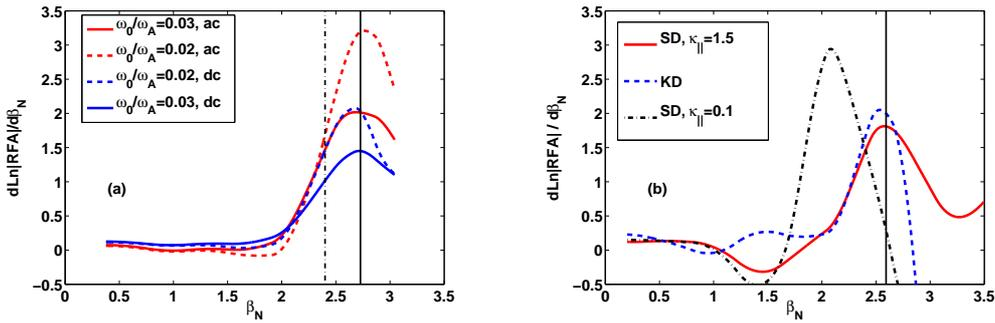
Figure 3: *Robustness of the logarithmic definition of the RFA threshold in predicting the no-wall beta limit. (a) Robustness against variation of the plasma rotation and the external field excitation frequency. (b) Robustness against the RWM damping models with strong damping.*
