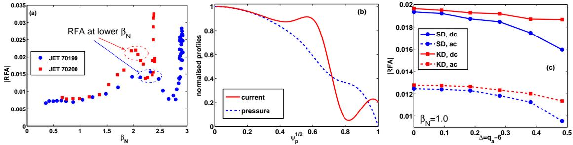
Figure 4: (a) The low-beta RFA response measured in the JET pulses. (b) The plasma equilibrium current and pressure profiles, re-constructed from the pulse 70200 and used in the peeling mode modelling. (c) The RFA response of the stable  $n = 1$  peeling mode with sound wave (SD) versus kinetic damping (KD) models, and dc versus ac excitations.
