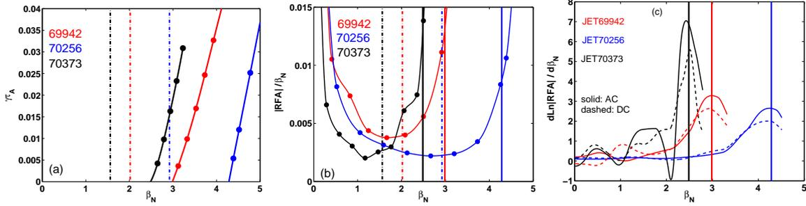
Figure 1: (a) Growth rates (solid) of the  $n = 1$  ideal kink mode versus  $\beta_N$  for three JET plasmas. The dash-dotted vertical lines indicate the corresponding  $n = 1$  RFA threshold measured in experiments. (b) The MARS-F computed RFA amplitude for these three plasmas. (c) Modelling shows that the logarithmic definition of the RFA thresholds match well the no-wall beta limit.
