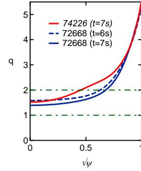
Figure 1: High- $\beta_N$  JET discharge limited by  $n = 1$  mode ( $B = 1.8T$ ,  $I_p = 1.2MA$ ,  $q_{95} = 5$ ,  $P_{tot} = 21MW$ ).
