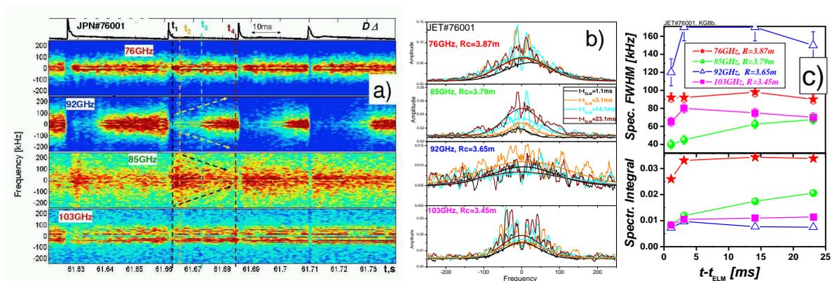
Figure 1: (a) Reflectometer spectrograms. (b) Fourier spectra for 4 consequent times between 2nd and 3d ELMs shown on (a). (c) FWHM and integral of spectra shown on (b).
