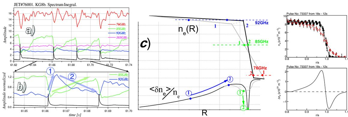
Figure 2: (a) Spectrum integral traces for 4 probing frequencies. (b) Different dynamics of "85" and "92" signals (normalized). (c) Model of  $n_e(R)$  and  $\frac{\delta n_e}{n_e}(R)$  evolution. (d) Experimental example of  $n_e(R)$  dynamics [7].
