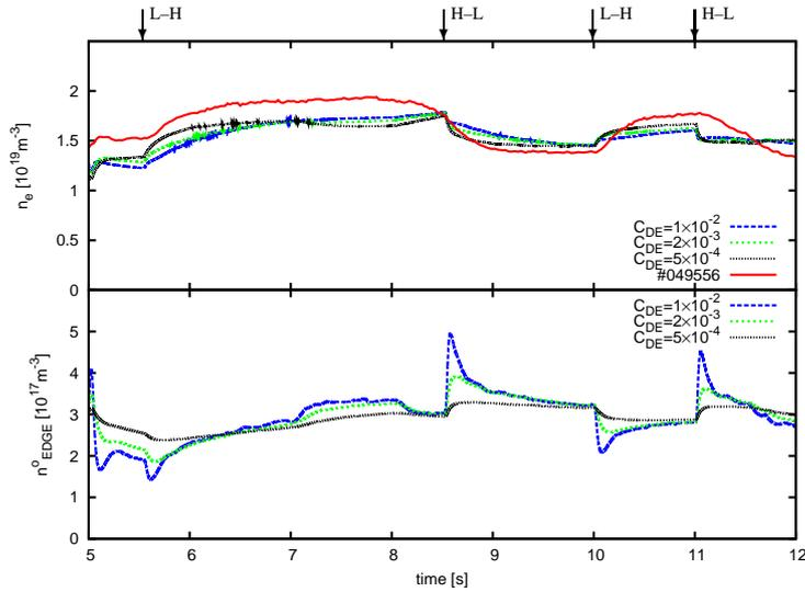
Figure 4: Line averaged density (top) and edge neutral density (bottom).
