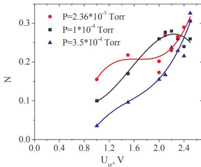
Fig. 6. Normalized plasma density as a function of generator anode voltage at different neutral gas pressures.
