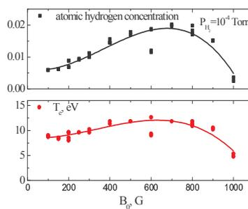
Fig. 4. Dependence of atomic hydrogen concentration and electron temperature on axial magnetic field.
