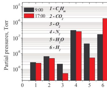
Fig. 7. Mass-spectrometer measurements of partial pressures before and after 6-hour RF discharge.
