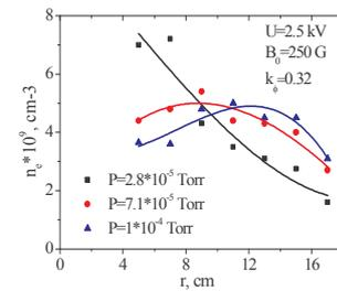
Fig. 5. Plasma density profiles for different neutral gas pressures.
