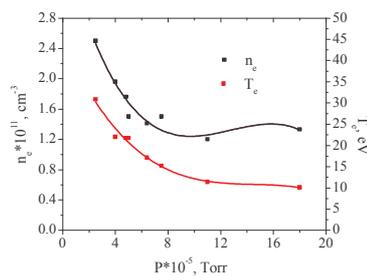
Fig. 8. Plasma density and temperature in combined discharge as a function of neutral gas pressure.
