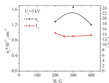
Fig. 9. Plasma density and temperature in combined discharge as a function of magnetic field.
