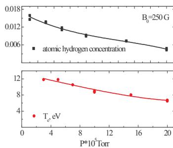
Fig. 3. Dependence of atomic hydrogen concentration and electron temperature on neutral hydrogen pressure.
