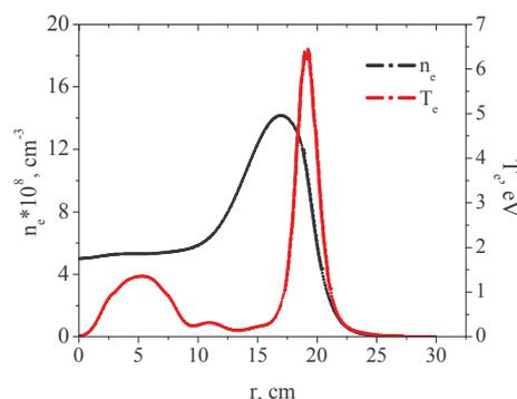
Fig. 11. Radial profiles of plasma density and temperature at time moment  $t=10^{-4}$  s (calculated).
