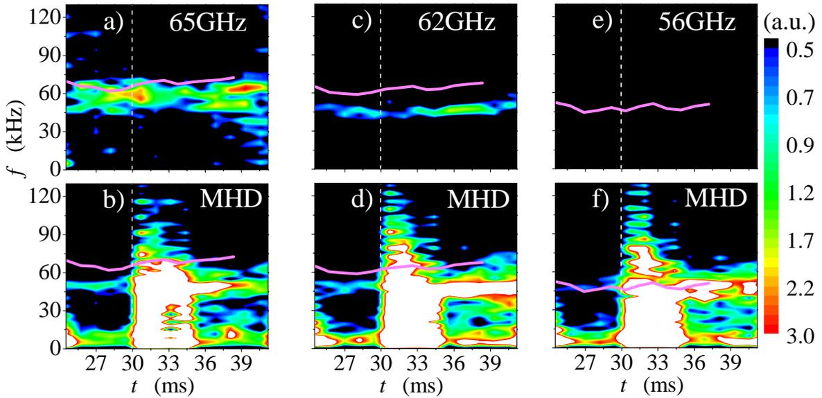
Fig. 5.  $f_D$  (a, c, e) and MHD (b, d, f) spectra for  $f_i = 65, 62, 56$  GHz.
