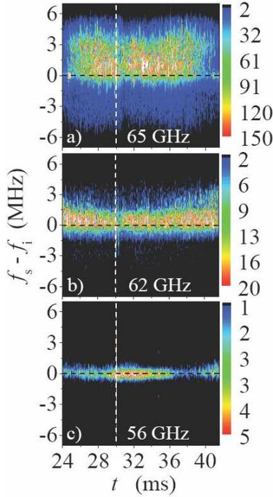
Fig. 2. ES Doppler shifted spectra for  $f_i = 65$  (a),  $62$  (b),  $56$  GHz (c).
