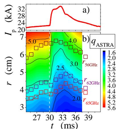
Fig. 1. Plasma current, UHR radial positions for  $f_i = 56, 62, 65$  GHz (squares) and the safety factor profiles obtained with ASTRA code modelling.
