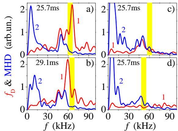
Fig. 4.  $f_D$  (1) and MHD (2) spectra for  $f_i = 65$  GHz (a, b),  $62$  GHz (c),  $56$  GHz (d).
