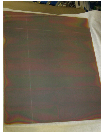
Figure 4: 600 mm x 720 mm PECVD \mu\text{cSi:H} layer from MAMELUK at 162 MHz.
