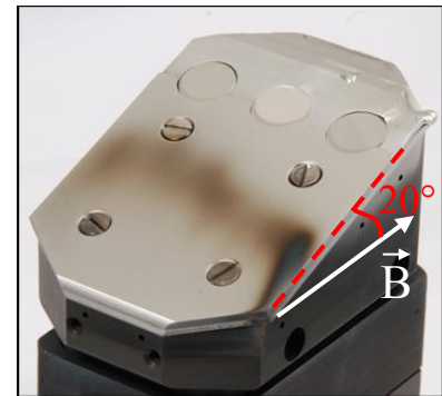
Figure 1. Test limiter with mirrors after exposure
