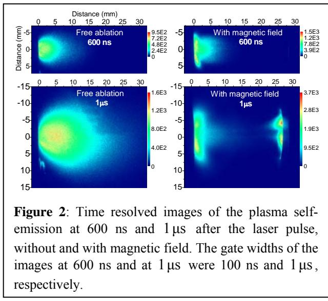
**Figure 2:** Time resolved images of the plasma self-emission at 600 ns and 1  $\mu$ s after the laser pulse, without and with magnetic field. The gate widths of the images at 600 ns and at 1  $\mu$ s were 100 ns and 1  $\mu$ s, respectively.
