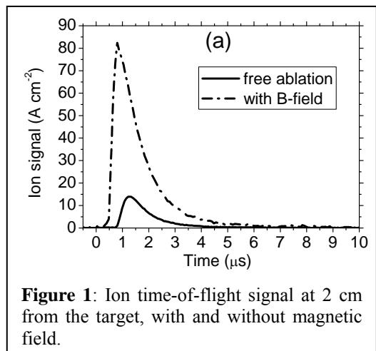
**Figure 1:** Ion time-of-flight signal at 2 cm from the target, with and without magnetic field.
