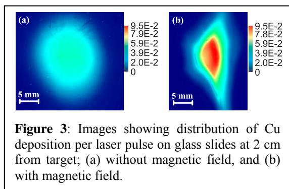
**Figure 3:** Images showing distribution of Cu deposition per laser pulse on glass slides at 2 cm from target; (a) without magnetic field, and (b) with magnetic field.
