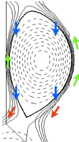
Figure 1: Magnetic drifts (vertical, downwards), Pfirsch-Schüter parallel flows (upwards near midplane), and divertor parallel flows (downwards, towards divertors)
