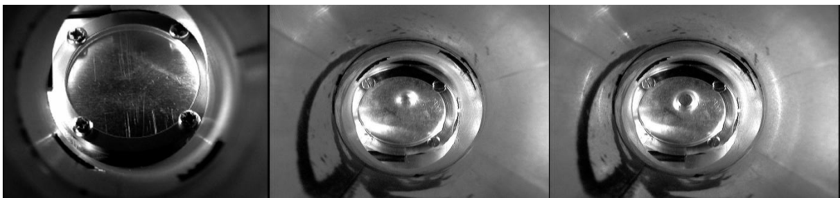
Fig. 3 – The impact of a pellet on the thin Al target, showing a very limited dispersion.
