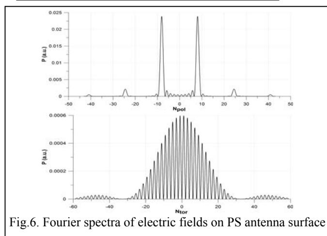
Fig.6. Fourier spectra of electric fields on PS antenna surface
