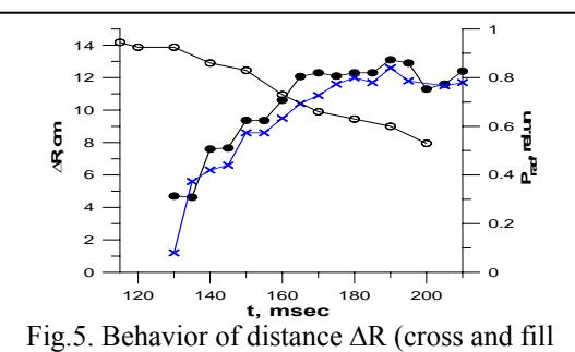
Fig.5. Behavior of distance  $\Delta R$  (cross and fill circles) and  $P_{rad}$  (empty circles) vs time
