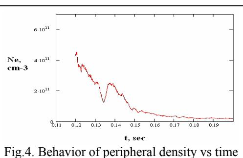
Fig.4. Behavior of peripheral density vs time
