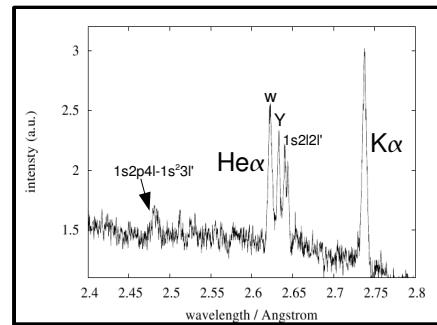
Figure 1: X-ray spectrum obtained from the irradiation of a 5  $\mu\text{m}$  thick Ti foil.
