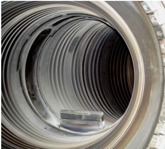
Fig.1. Lithium limiter with the collector plates in the T-11M.
