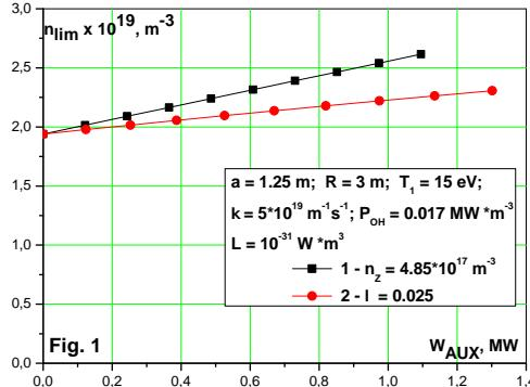
Figure 1: Critical plasma density as a function of auxiliary heating power for cases I and II, i.e. impurity ions density independant and proportional to the main plasma density.
