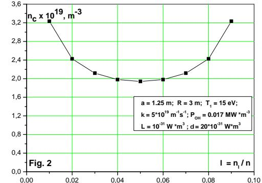
Figure 2: Critical plasma density as a function of the coefficient of proportionality between impurity ions density and main plasma one, for the case III of feedback system usage.
