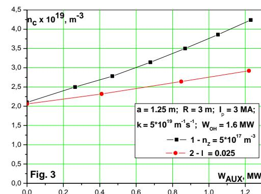
Figure 3: Critical plasma density as a function of auxiliary heating power, ASTRA modeling.
