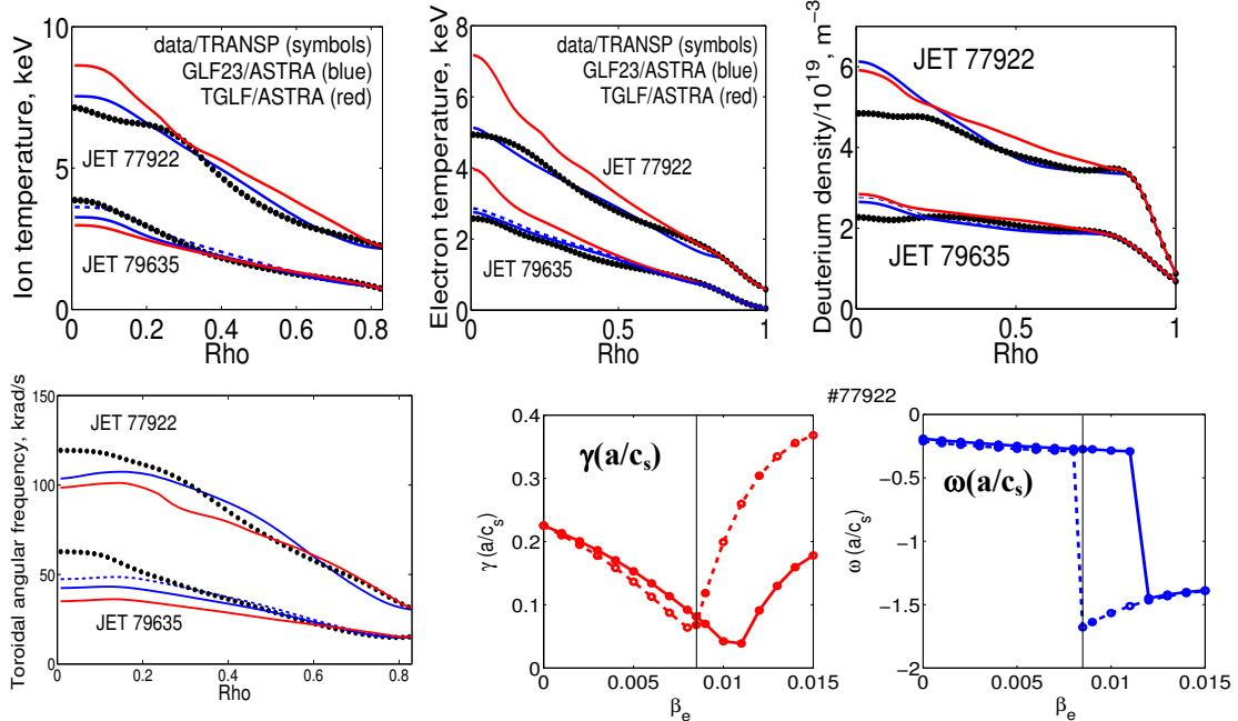
Fig. 3. Simulations with GLF23 and TGLF models performed with  $\alpha_E=0.5$  and  $Pr=0.5$  (solid curves) for JET HS. Dashed blue curves show the GLF23 simulations performed with  $\alpha_E=1$  for low power
