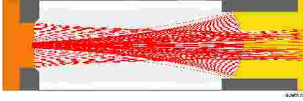
Fig. 1. Simulation of an electron beamlet in a single diode aperture. The left side is the cathode with a cathode plasma, the right one is the anode with a stream of plasma. Diameter of the cathode aperture is of 3 mm, anode one is 4.4 mm, the diode gap is 12 mm, the voltage is 100 kV, the electron current density averaged over the cathode aperture is 63 A/cm 2 , the ion current density at the anode is ~1 A/cm 2 , the diode current is 1.1 kA. The maximum pitch angle of electrons is ~0.07 rad. The magnetic field is 0.05 T.
