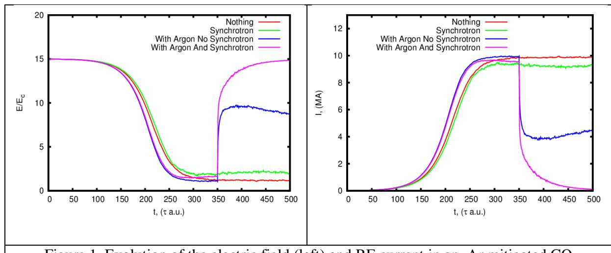
Figure 1. Evolution of the electric field (left) and RE current in an Ar mitigated CQ
