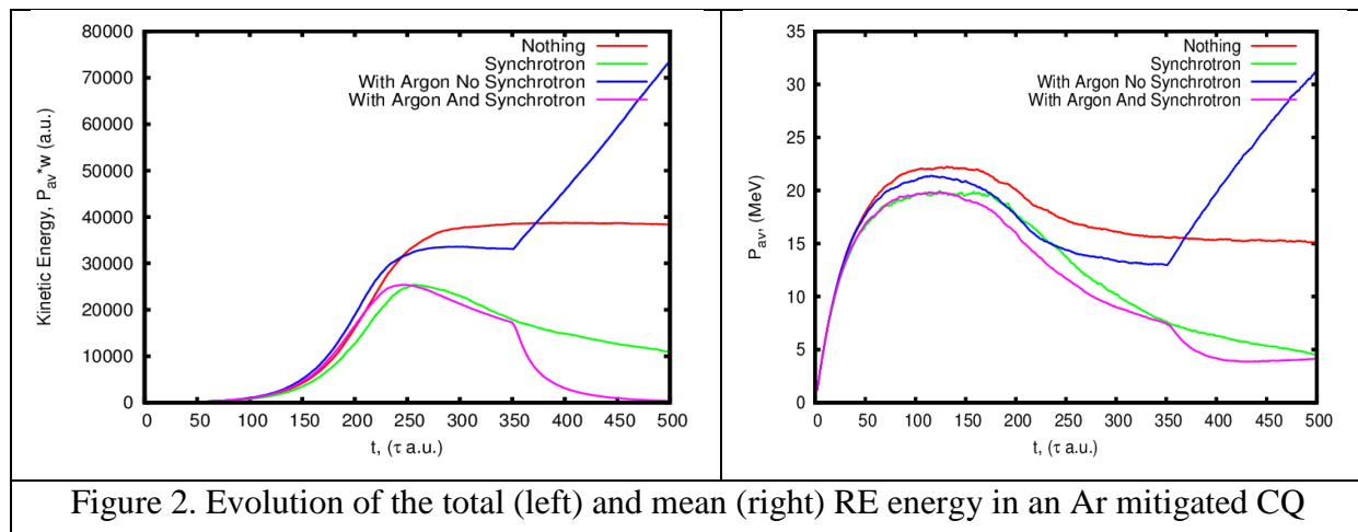
Figure 2. Evolution of the total (left) and mean (right) RE energy in an Ar mitigated CQ
