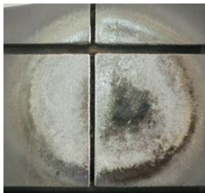
Fig. 4. Fragment of mock-up after irradiation with plasma gun; 100 Shots; 0.7 \text{ MJ/m}^2 ;
