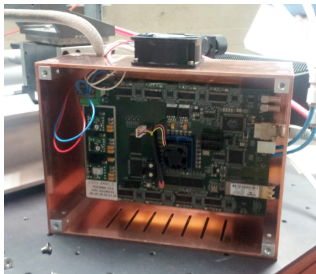
Figure 1 The mother board FPGA based coupled with the GEM detector
