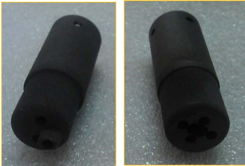
Fig. 1: Two graphite probe heads for EAST with 3 cm diameter each and overall lengths of 10 cm, here shown without the probe pins inserted.
