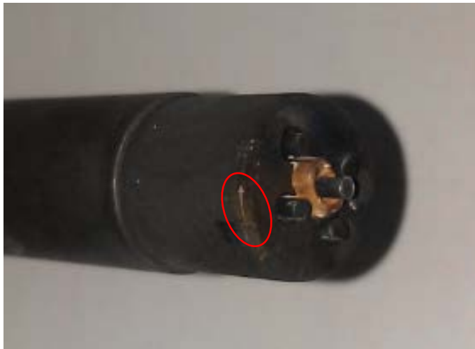
Fig. 3: The five pin probe head with the spot where the UNCD-coating dropped off marked. A SEM of this spot is shown in Fig. 4.
