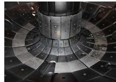
Fig. 8. W tiles in low divertor of the Globus-M tokamak
