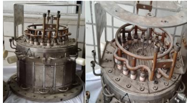
Figure 2 arc discharge chamber with 20 lists of magnets, 21 cm long
