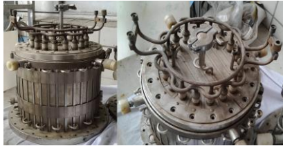
Figure 1 arc discharge chamber with 36 lists of magnets, 24 cm long
