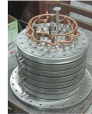
Figure 3 arc discharge chamber with 7 turns of magnets, 21 cm long
