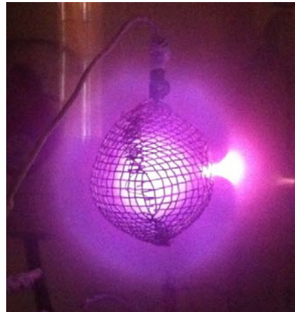
Fig. 2: Complex space charge structure inside and around a grid cathode with a hole
