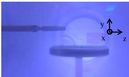
Figure 1: The cylindrical Langmuir probe in an Argon plasma in ALINE. The radio-frequency antenna is the disc seen in the.
