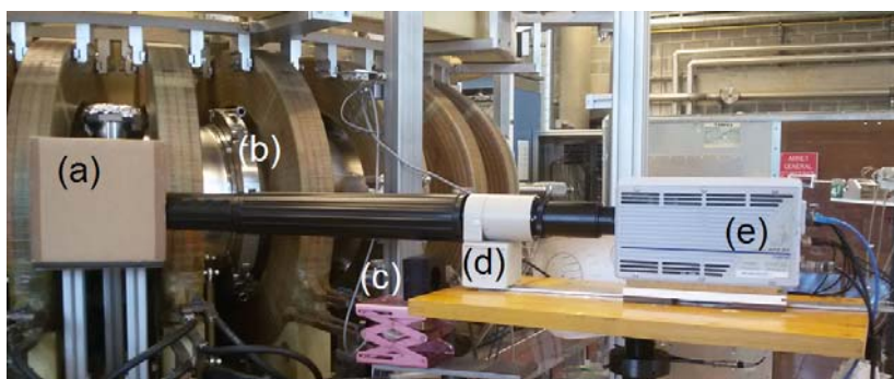
Figure 2: Imaging system and its different components. (a) Dark box with mirrors to improve the view angle on the coating. (b) TORPEX vacuum vessel and toroidal magnetic field coils. (c) Configurable optical passband filter on movable arm for easy insertion and removal. (d) Image Intensifier Unit. (e) FastCam.
