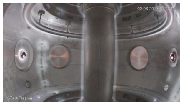
Figure 3: Top MC coil fired into a glow discharge during pulse #2502. The peak current in the coil was 420kAt, resulting in \sim 40 loop volts at the coil, and visible breakdown filaments on the coil.
