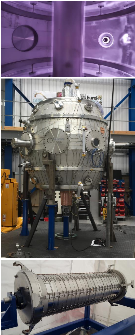
Figure 1: Glow discharge in ST40 (top), the current state of construction (middle), and the central tube assembly (bottom) with magnetic diagnostics.
