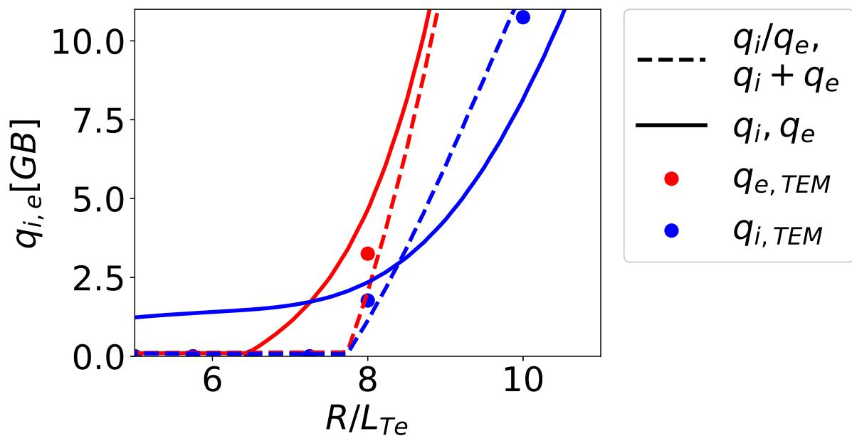
Figure 1: An example of threshold mismatch. One can see the two different styles of neural network fits. Dots are QuaLiKiz output, and the solid lines represent a fit directly on flux. The dashed line is a fit on  $q_i/q_e$  and  $q_i + q_e$ . Ions in blue and electrons in red. Note the exact match of threshold with the dashed lines.
