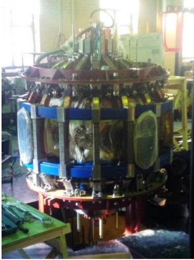
Fig. 1. The trial assembly of Globus-M2.
