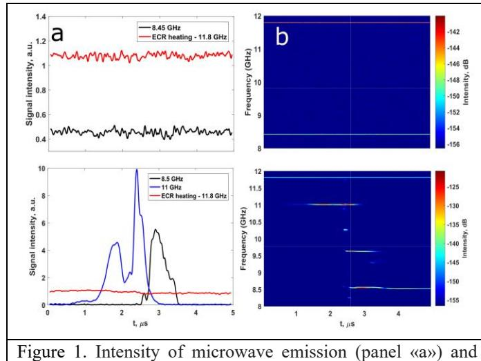
Figure 1. Intensity of microwave emission (panel «a») and dynamic spectra of plasma emission in 8-12 GHz range (panel «b») to the generation of cw emission (upper plot) at  $B_{\min}/B_{\text{ECR}} = 0.947$  and periodic bursts (lower plot) at  $B_{\min}/B_{\text{ECR}} = 0.935$ . Stray radiation of the heating TWT amplifier at 11.8 GHz is shown with a red line.
