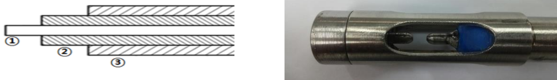
Fig. 2 Plasma discharge probe concept (left) and probe manufactured (right)
