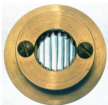
Fig.1. Ionizer of "blinds" type
