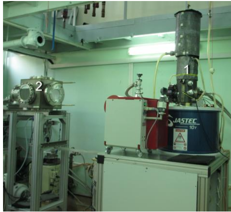
Fig.1. Experimental setup. 1 – 250kW@250 GHz gyrotron. 2 – Discharge chamber.
