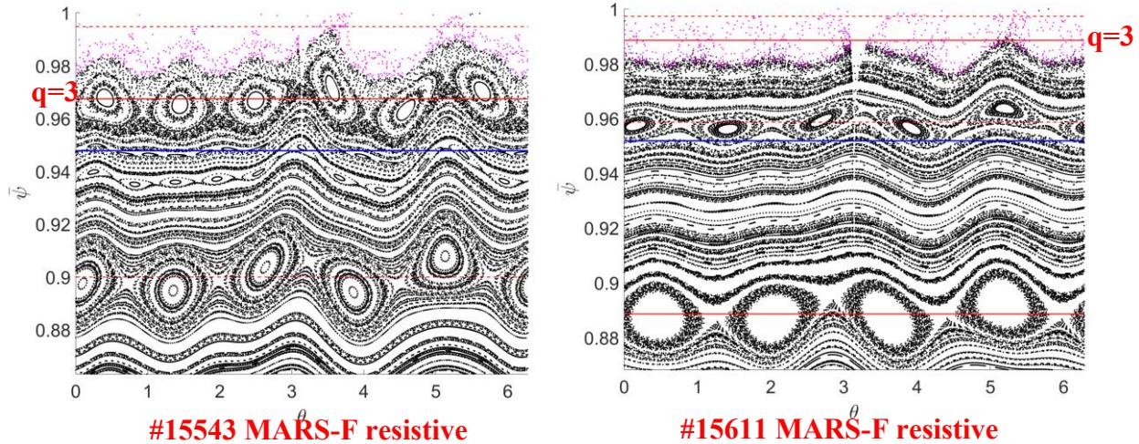
By evolving slow D ion markers along the field lines, we can trace the field in the poloidal plane. The figures compare the perturbed field as obtained from the resistive plasma response in the case of two pulses. It seems #15543 does not resonate because @ $q=3$ , no stochastic losses (magenta dots) occur. In #15611, the  $q=3$  flux surface is in the same location as the pedestal, thus allowing for the coils to affect the MHD through significant losses.
