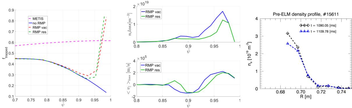
The losses after 8ms of simulation in EBdyna\\_go are shown above in the figures (left and middle). On the experimental side, a drop of density at the top of the pedestal is measured (right plot). Furthermore, we find experimental evidence of a change in bulk plasma rotation through the decrease of the (1,1) mode frequency as estimated by the Mirnov coils.
