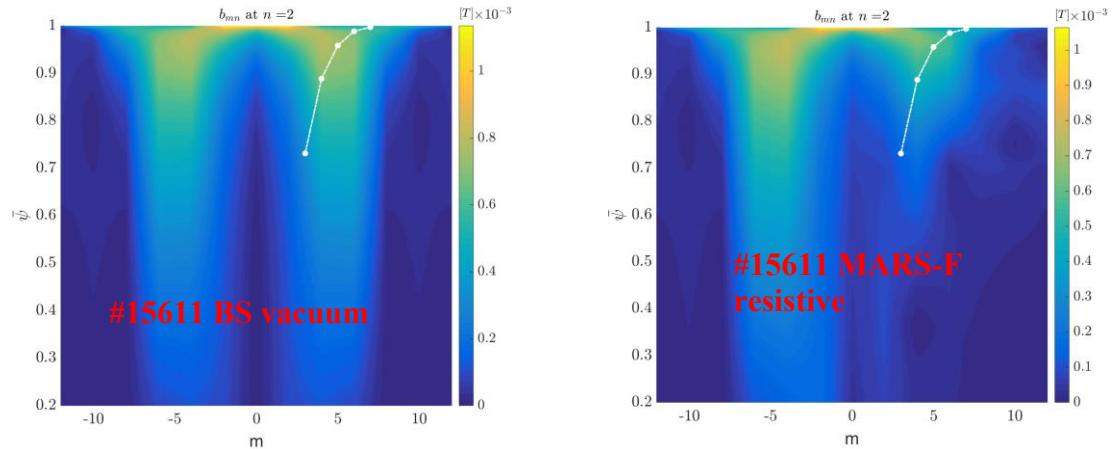
The radial perturbation generated by the RMP coils is analysed through the Fourier transform of the plasma response (figure above) and we only consider the main harmonic  $n=2$ , neglecting the impact of further sidebands.
