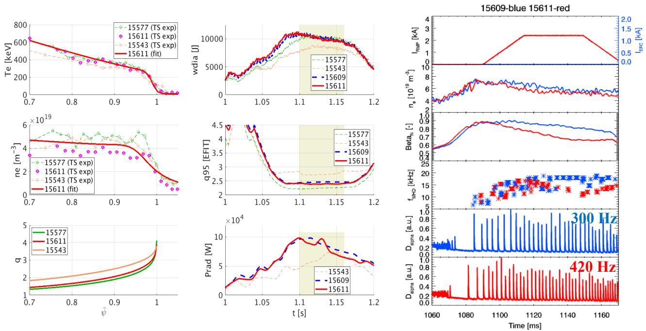
HFS RMP triggers no significant energy loss (wdia) and a moderate density pump-out in the edge region, whilst still able to modify  $f_{ELM}$  and  $n_e$  pedestal height. Only the configuration in #15611 is triggering a measurable change in plasma behavior.
