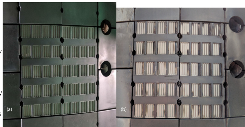
Figure 4: Mockup antenna installed on the high field side of DIII-D (a) before and (b) after the run campaign.
