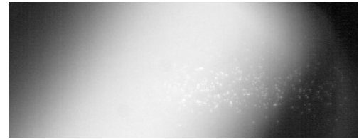
Figure 2: Phantom camera image of multiple 3.25 \pm 1.0 \mu m radius dust grains emitting thermal radiation after exiting the plasma column, B = 0.4 T .
