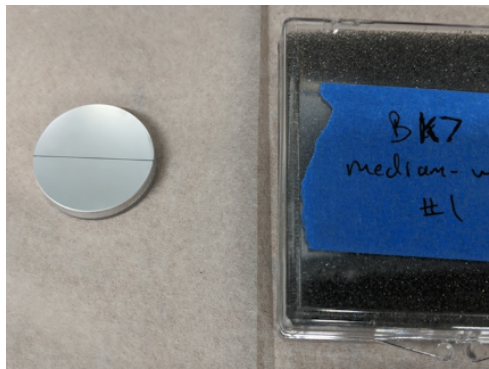
Figure 1: Phase plate fabricated by masking a one inch diameter NBK-7 substrate with a flat ribbon 0.254 mm wide.
