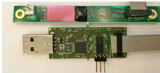
Figure 2: PH32 chip with SURE (Simple USB Readout Equipment) data acquisition card. The ASIC is hidden by a layer of epoxide to protect sensitive wire bonds.
