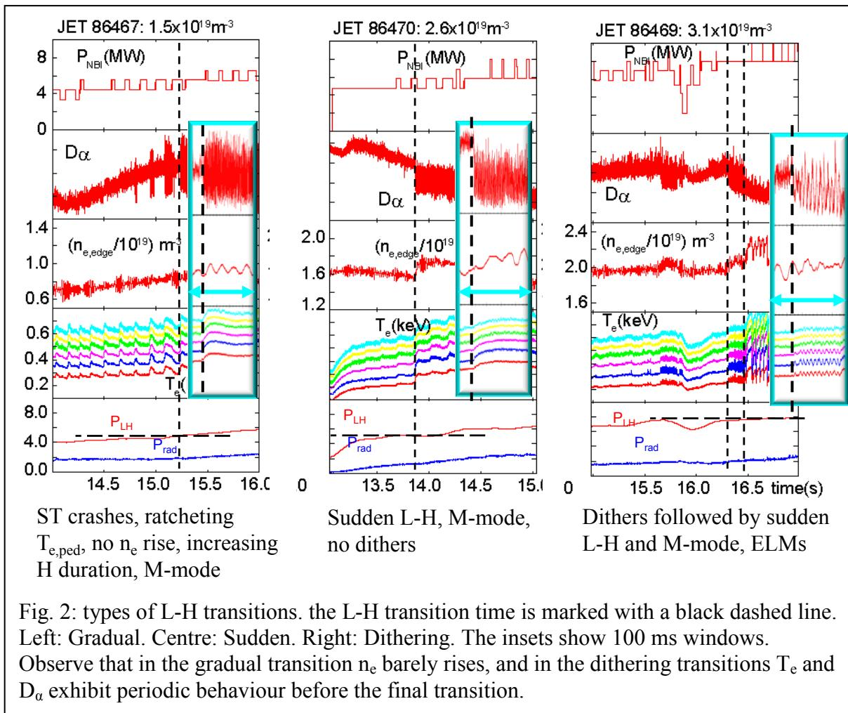
Fig. 2: types of L-H transitions. the L-H transition time is marked with a black dashed line. Left: Gradual. Centre: Sudden. Right: Dithering. The insets show 100 ms windows. Observe that in the gradual transition  $n_e$  barely rises, and in the dithering transitions  $T_e$  and  $D_\alpha$  exhibit periodic behaviour before the final transition.
