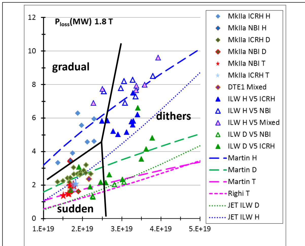
Fig. 3:  $P_{\text{LH}}$  for various L-H transition experiments at 1.8 T in JET. The black solid lines delimit the types of L-H transition: gradual, sudden and dithering.
