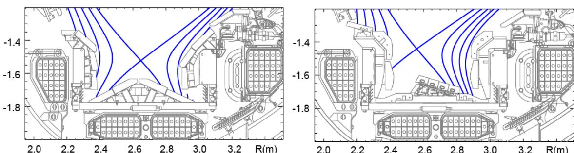
Fig 1, left: divertor and separatrix geometry of the JET-C divertor, MkIIA, during H, D, T, D+T campaigns in 1997. Divertor tiles were CFCs.
