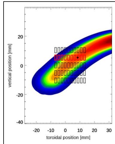
**Figure 3:** Modelled ion beam distribution at the detector plane with the 5 x 10 channel detector matrix, aligned best to shot #17747 data.
