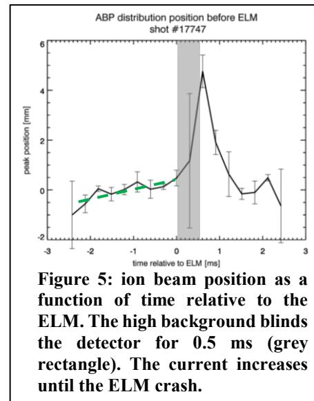
**Figure 5:** ion beam position as a function of time relative to the ELM. The high background blinds the detector for 0.5 ms (grey rectangle). The current increases until the ELM crash.
