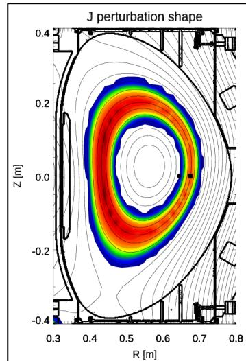
**Figure 2: Current perturbation shape in the simulation. The 3 points on the LFS mid-plane show the boundaries of the perturbation.**
