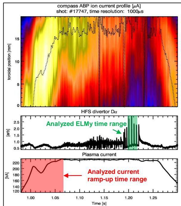
**Figure 4:** Ion beam distribution on a row of the ABP detector array (a) with the fitted maximum positions (dotted line), HFS divertor  $D_\alpha$  (b) and plasma current (c) signals as a reference.
