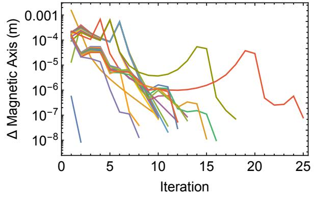
Figure 1: *Inner loop convergence of the magnetic axis.*
