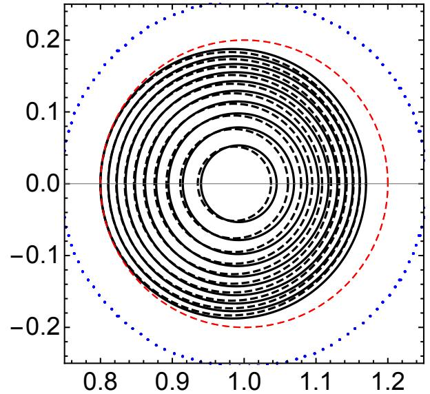
Figure 2: The equilibrium shifts to the left over the course of the simulation. The solid flux surfaces are the initial equilibrium and the dashed surfaces are the final.
